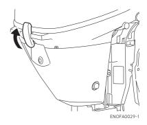
Remove starter lock cable from recoil starter by loosening the screw for the starter lock cable.
