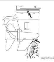
Install the upper oil plug, and then remove oil tube nozzle and install the lower oil plug.
