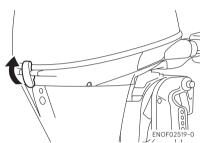
2. Remove starter lock cable from recoil starter by pulling the starter lock cable.
