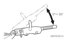
Angle of Multi-Function Tiller Handle according to the number of spacers.
