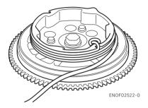
5. Tie a loop in the another end of the emergency starter rope and attach socket wrench, Both the loop and the wrench are provided in outboard motor box.
