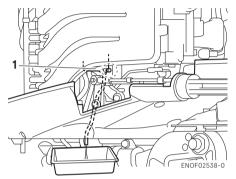
1. Vapor separator drain screw
